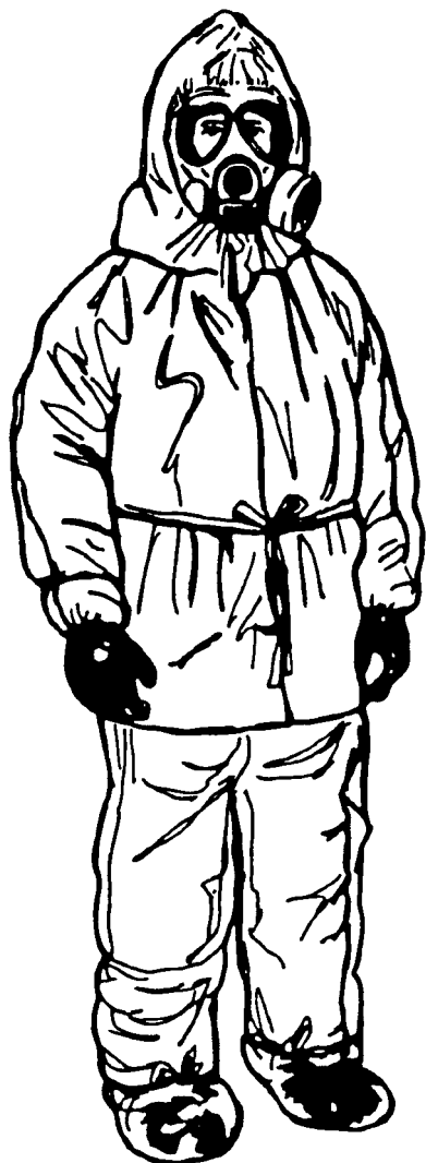
Figure 1-3. Contamination avoidance and liquid protective suit.
